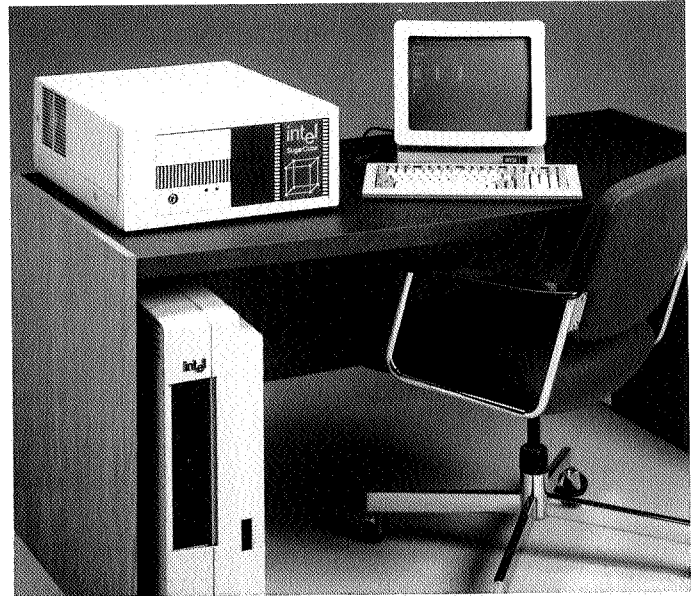
Intel SugarCube™ systems consists of the Cube Manager (bottom left), user terminal, and Cube (top left), which provides the computing power of 4 or 8 processing nodes.
